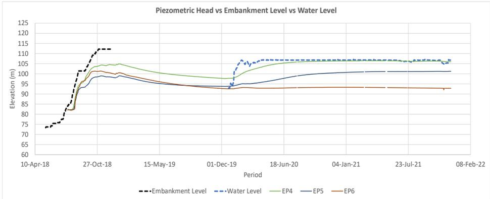
**Figure 6: Piezometer monitoring data (piezometer elevation +82.59 m)**
