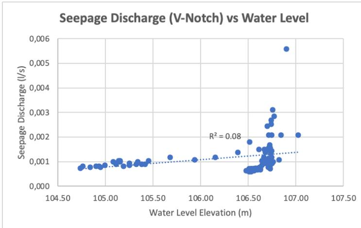
**Figure 11: V-Notch Data versus Reservoir Water Level**
