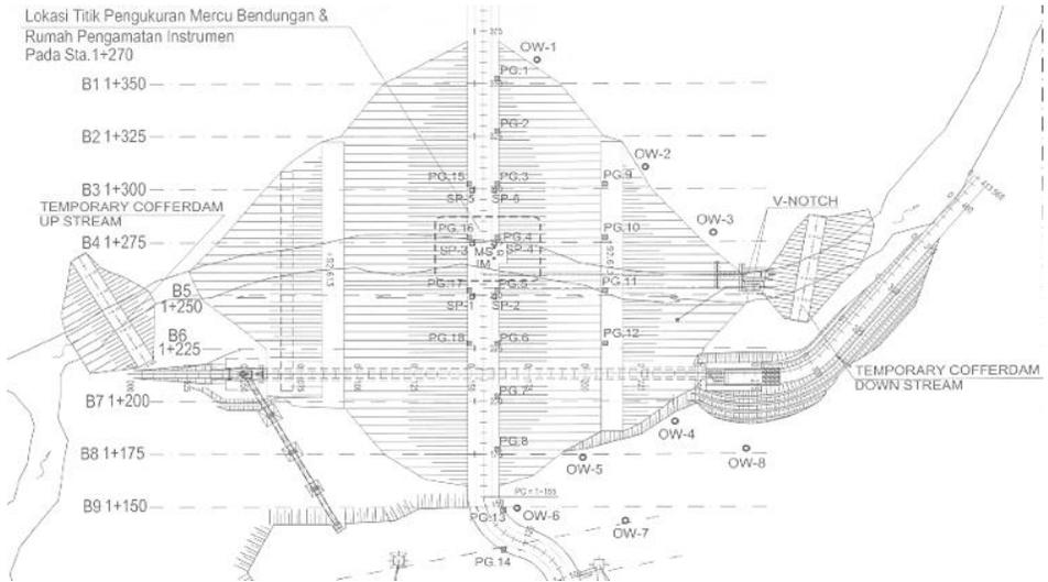
**Figure 12: Installation Layout of Observation Wells (coded OW-)**
