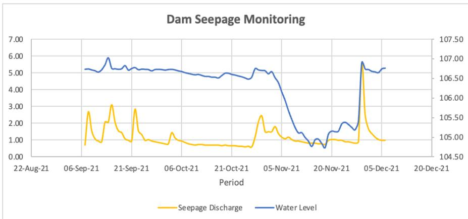
**Figure 10: V-notch Monitoring Data**
