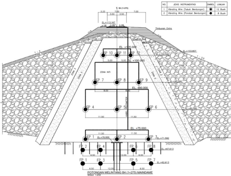
**Figure 3: The placement layout of the piezometer in Sindang Heula Dam**
