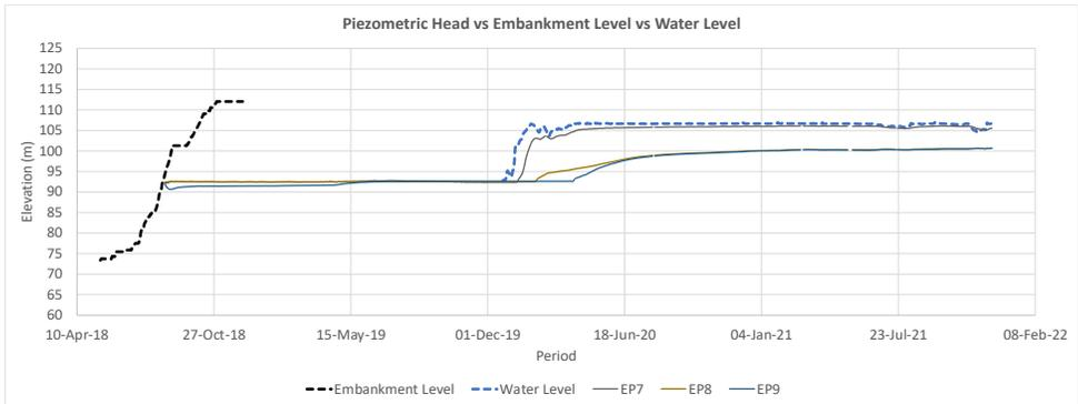
**Figure 7 Piezometer monitoring data (piezometer elevation +92.59 m)**
