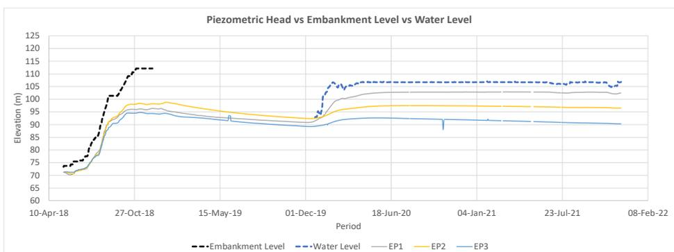
**Figure 5: Piezometer monitoring data (piezometer elevation +71.59 m)**
