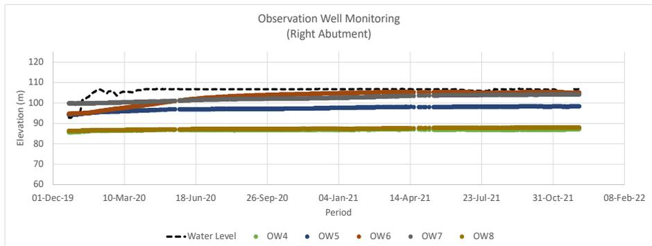
**Figure 14: Observation Well Monitoring Data (Right Abutment)**
