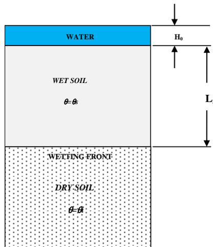
**Figure 1 : Green-Ampt model:  $L_f$  Depth to wetting front,  $\theta$  water content**
