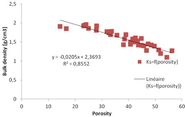
**Figure 9: The bulk density expressed in function of the porosity**
