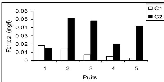
**Figure 13:** Space variation of the Iron values on the level of C1 and C2.
