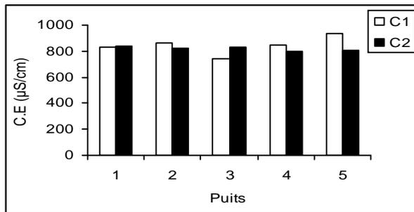
**Figure 4:** Space variation of the values of electric Conductivity (EC) on the level of C1 and C2.
