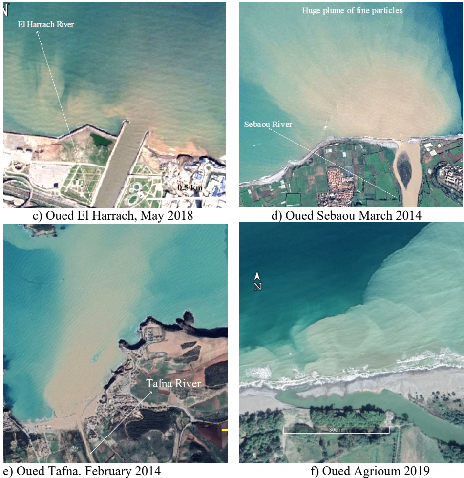
Figure 9: Some examples of the extent of fine particle discharge from Algerian Rivers into the sea (Google Earth)
