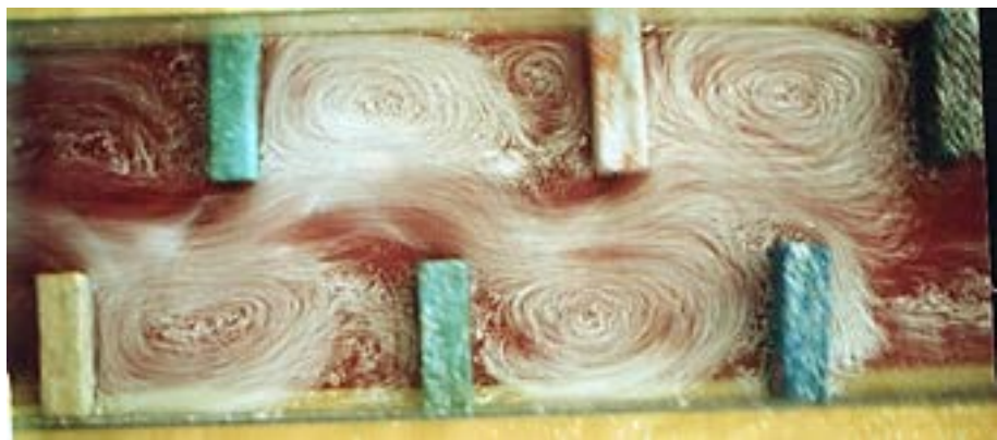
Figure 36: The chicane shape of the obstacles in a wadi is the best arrangement to accelerate the recharge of the alluvial aquifer (Photo Remini, 2004)
