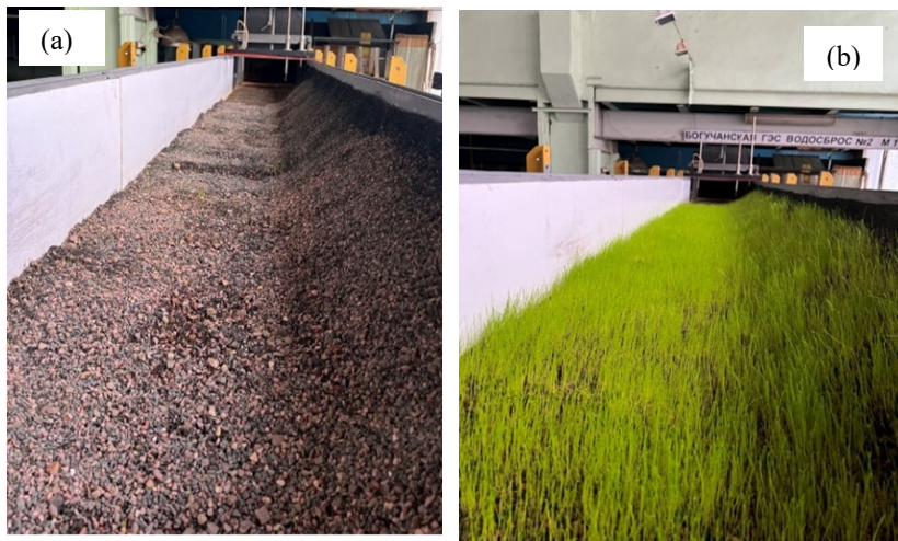
Photo 3: Options for protective coverings, (a) geomat with gravel filler; (b) geomat with vegetation. (Photo by Zhukova, 2024)
