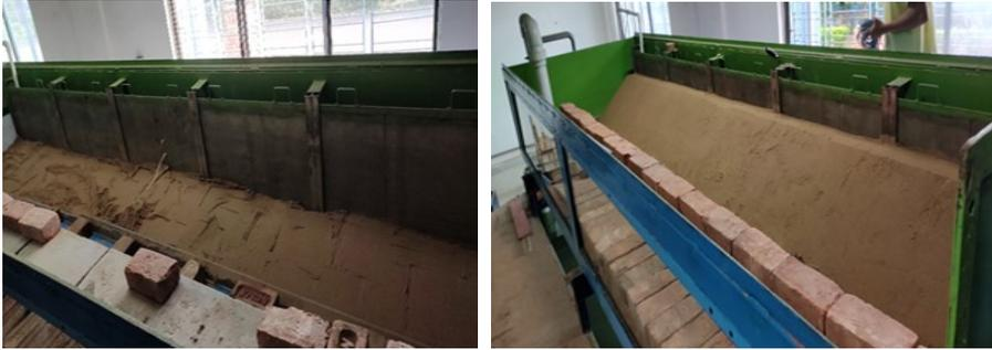
**Figure 3: Model Bank prepared in flume**
