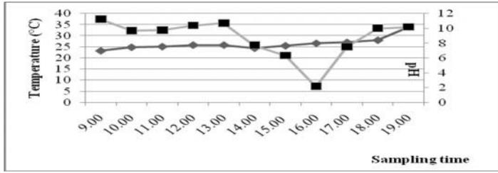
**Figure 1:** Evolution of daily temperature and pH of industrial wastewater collector.
